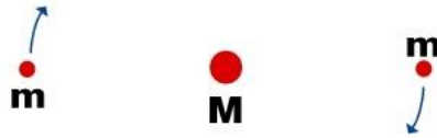
Figure 5 — Euler's "Counter-Earth" configuration. Two identical masses m in orbit around mass M in identical orbits 180^\circ apart
